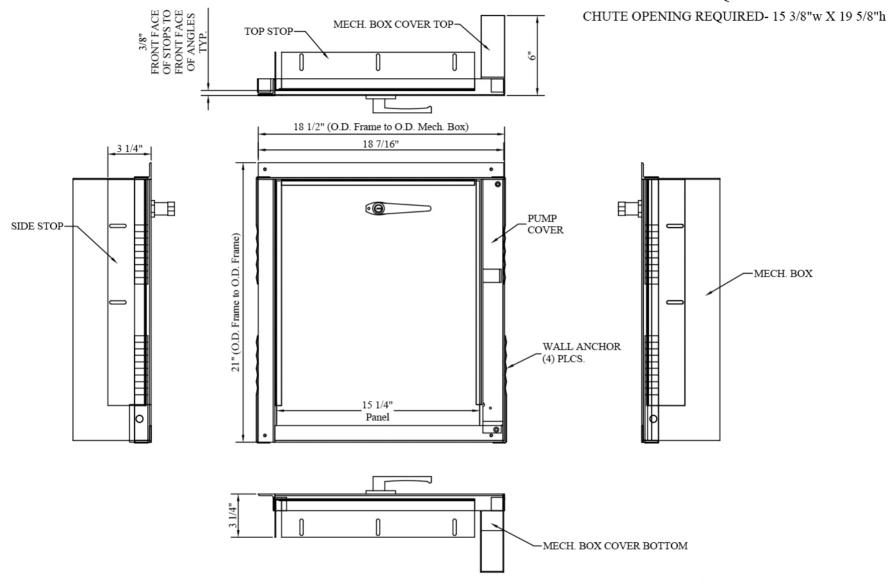
15"x18", bottom hinged, hand operated, self-closing intake door with 22 ga. SS front & 18 ga Al-Stl door back.
